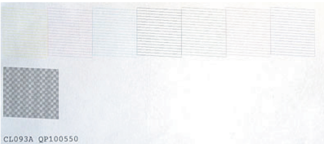
This is the usual printhead test plus a checkerboard pattern to further allow you to see if a printhead is clogged.
